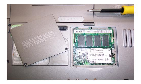
Most laptops will have an easily accessible hatch held in with screws in the middle of the back. This is where you'll find the RAM.
