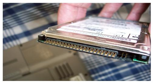
At one end is a row of teeth – these are how data moves to and from the hard drive. These are different for different types.
