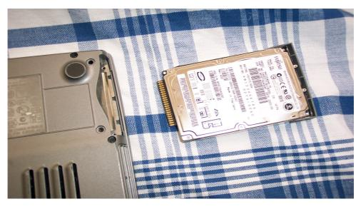
Once pulled out and turned over you can see that this hard drive has a label on it. This will tell you what kind of hard drive it is, how fast it is and how large. You will need to take the hard drive out of its caddie to replace it.
