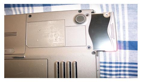
Undo the screws holding it in place. In this hard drive's caddie (its container) there are ridges to help you pull it out.
